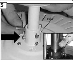
Insert downrod into yoke on top of the Fan Body. Align the hole in the Downrod with the hole in the Yoke. Insert the Pin through the Yoke and Downrod until the point appears on the other side. Install the Keeper Pin
